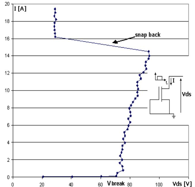
Figure 5. I - V trace for 100ns pulses
