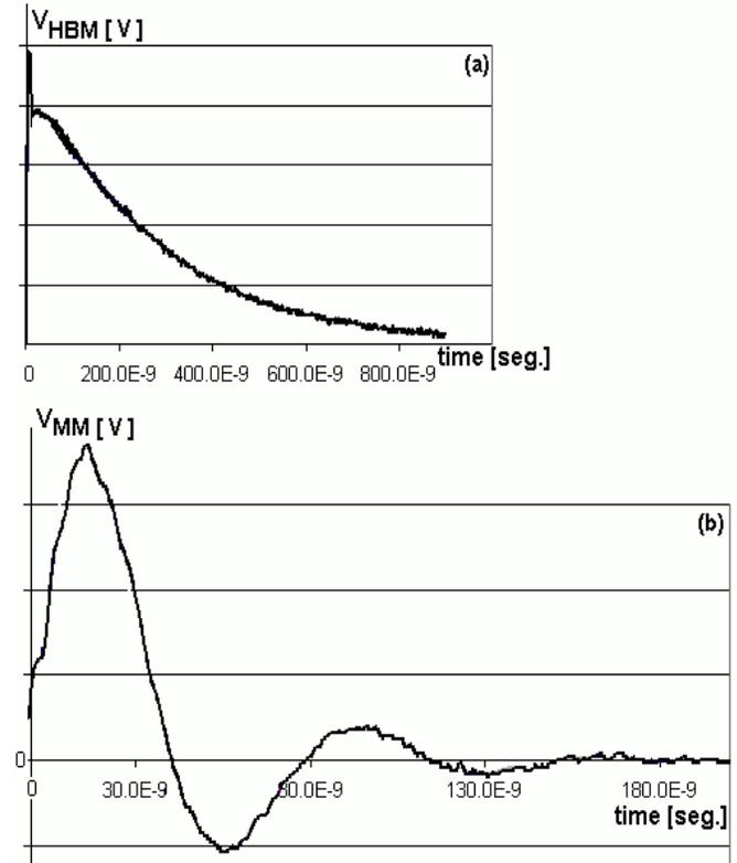
Figure 8. (a) HBM waveform modified. (b) MM waveform used.
