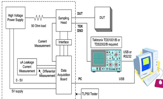
Figure 3. TLP50 block-diagram
