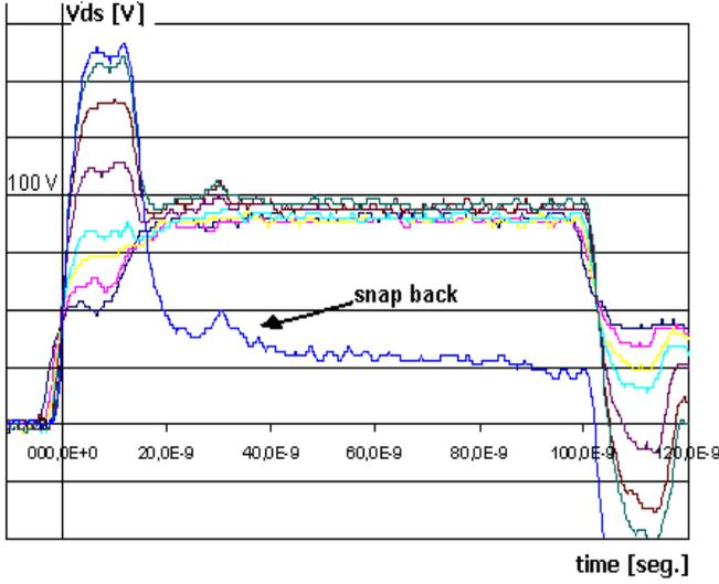
Figure 6.  $V_{ds}(t)$  for 100ns growing pulses
