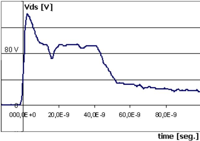
Figure 7.  $V_{ds}(t)$  breakdown for 200ns pulse
